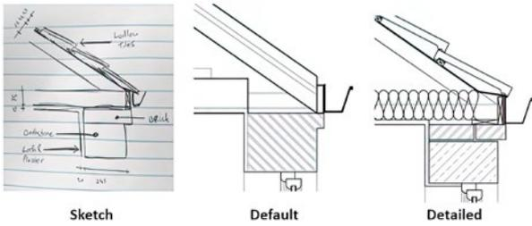
The reason I developed my graphical model this way was to limit the amount of overall modelling that I needed to do. I am a firm believer of modelling as efficiently as possible. For example, to limit the amount of modelling I need to do for my roof I have set a number of informal 'volumes' within the roof itself using Revit's built-in system family layering function:
