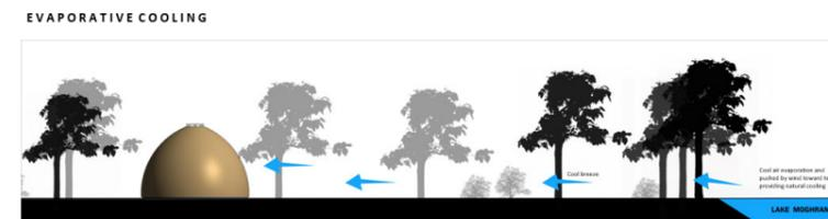
The site is in close proximity to Lake Moghran, the air around it will be significantly cooler than other locations. As a result, the cool air can be pushed by the easterly winds providing a slightly cooler breeze towards the tent. This could potentially help reduce mechanical cooling loads in the summer period.
