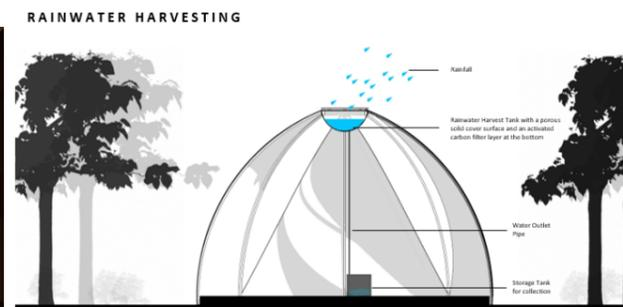
The design maximises an increase in rainfall during the winter period in Dubai by making use of a Rainwater harvest system at the top of the structure which captures rain and stores it in a tank/bottles through an outlet pipe. Water is filtered for drinking or any other use.
