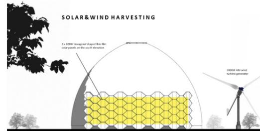
The proposal makes full use of the solar radiation in the location by using thin film panels on the South facing elevation which is highly exposed to heat gains from the sun as well as a wind turbine to harvest the strong winds in the area and help meet the energy load demands
