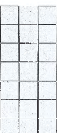
Figure 4 Full block stack bond using grooved block
