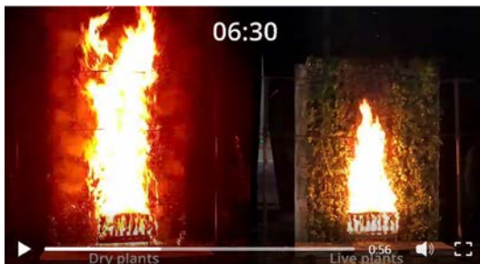
Snapshots of videos captured at 6 mins and 30 secs after initial ignition, showing the difference between dry plants (left) and live plants (right).
