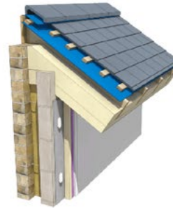
DL-358 Typical mono-pitch ridge to cavity wall detail - refurbished slate roof - insulation between and under rafters
