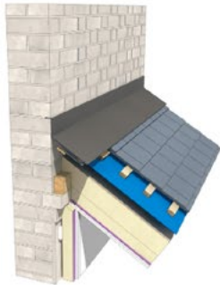
DL-353 Typical parly wall / solid masonry wall to lean to vented abutment detail - refurbished slate roof - insulation between and under rafters
