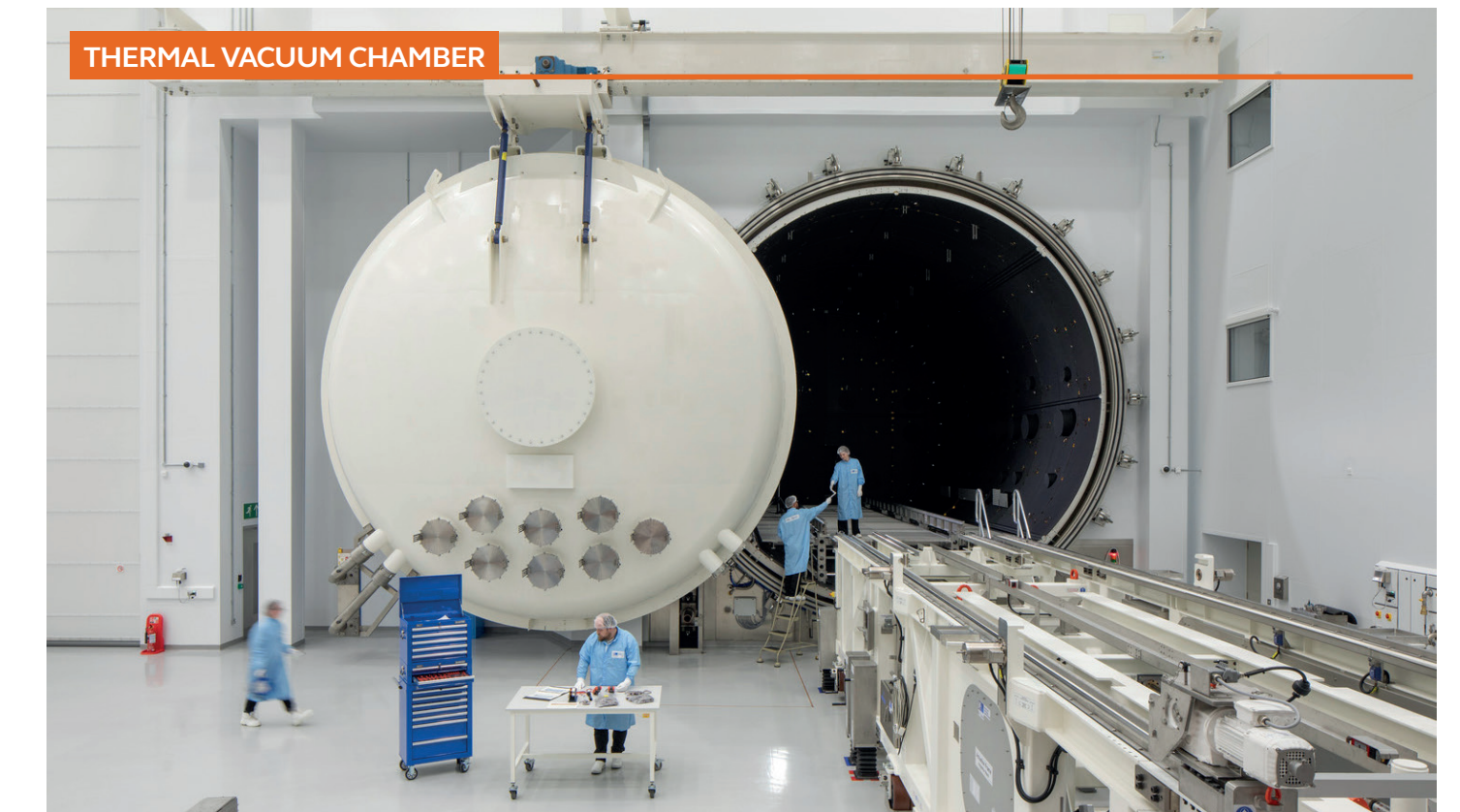
▲ Simulates a satellite's travel in conditions of space
