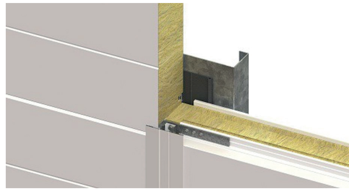
▲ Reusable - Recyclable - Airtight. Well-insulated aluminium composite panels carefully details to minimise structure
