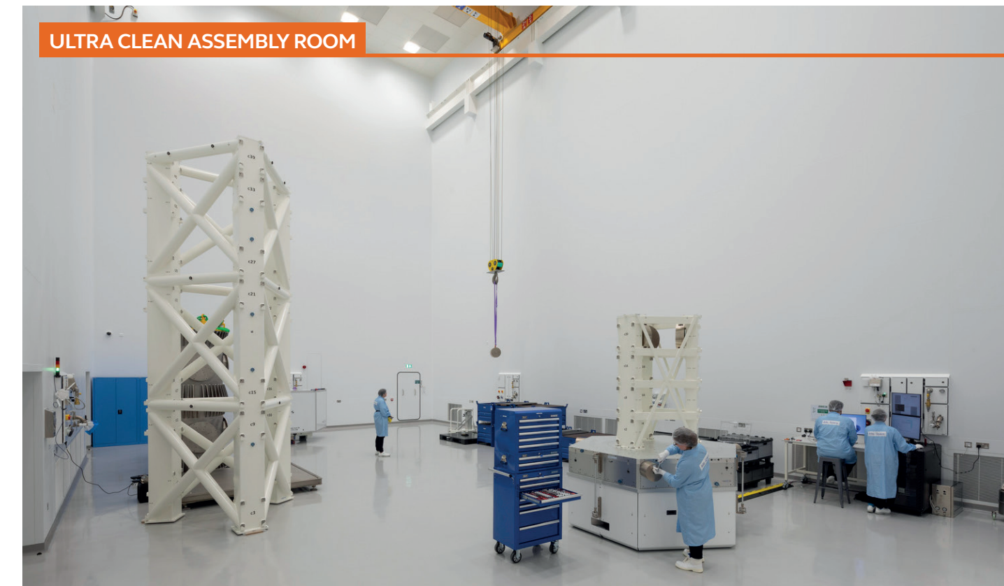
▲ ISO6 ultra clean testing space - Centre of gravity and component testing
