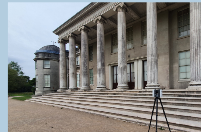
Using a Leica RTC360 laser scanner
