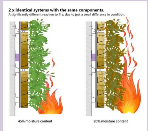
For designers, it is important to understand that the reaction to fire of a living wall system can be impacted by local environmental conditions such as dry weather and wind. As the moisture levels are reduced, so does any protection that this gives against fire spread.
