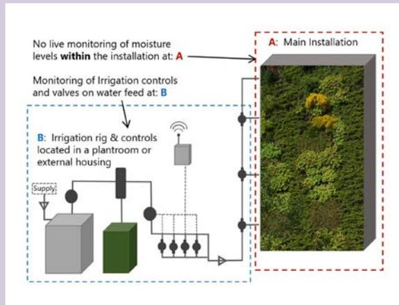
While a potential issue with a leaking, damaged pipe or blockage may be flagged up by a pressure drop indication when using this method, there is not an accurate method being applied to most installations to constantly monitor the wall itself, within the plant modules. This should happen at location (A) to confirm an actual moisture figure, (%MC) which is a clearly determined stipulation of the validity of the supporting FEA document.
