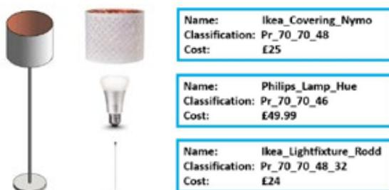
With this in mind, I have opted to model each item separately and create an 'assembly'. If you are not sure what an assembly is, it is a method of grouping objects into a schedule-able component made up of a number of individual components, if you will components within components. Once set up it allows each assembly to be recorded when I export my information into COBie.
