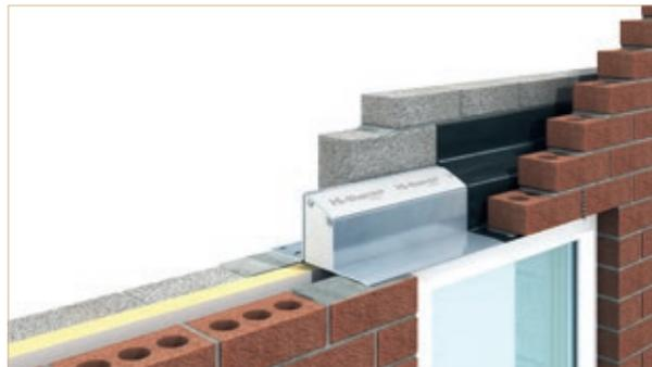
For instance, hi-therm+ lintels use a patented combination of a polymer isolater and galvanised steel. The polymer section provides a powerful thermal break in the lintel and significantly reduces its conductivity value, with a psi value of between 0.03 and 0.06 W/m.k. As a result hi-therm+ lintels are up to five times more thermally efficient and are also available in the same lengths, sizes and loading capacities as the standard range of lintels.
