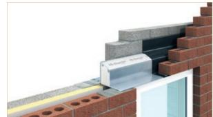
For instance, hi-therm+ lintels use a patented combination of a polymer isolater and galvanised steel. The polymer section provides a powerful thermal break in the lintel and significantly reduces its conductivity value, with a psi value of between 0.03 and 0.06 W/m.k. As a result hi-therm+ lintels are up to five times more thermally efficient and are also available in the same lengths, sizes and loading capacities as the standard range of lintels.
